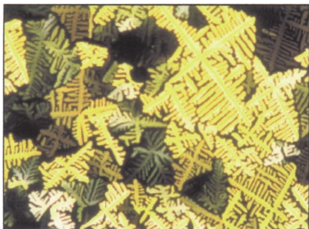
Figure 2. Representative optical polarized micrograph ( 100\times ) of texture exhibited by a body-centered tetragonal micellar mesophase of 1 at the transition from the isotropic liquid state at 220^{\circ}\text{C} .
